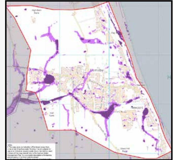
Figure 08: CDA 008: 1 in 200yr depth surface flooding risk
